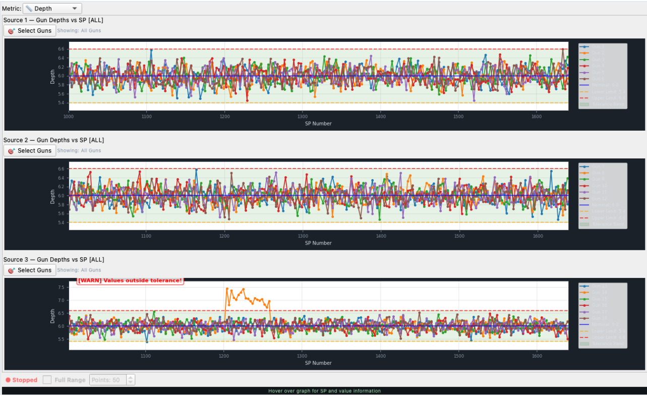
Figure 14. Live trend graphs — gun depth against shot point for three sources, with the tolerance band shaded and a gun drifting out of tolerance flagged on source 3.
